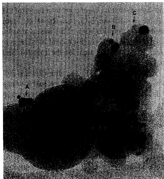
Fig. 3. The TEM photograph (magnification of 800,000) of Imp-Rh-Sn/SiO 2 (Sn/Rh = 0.40).
